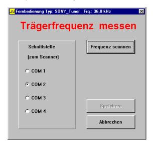
Please set here the interface were the IR-scanner was connected. After the actuation of the button "frequence scan" the following window appears.
