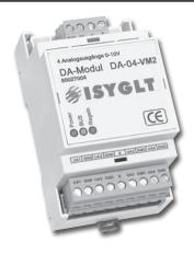
The voltage outputs are galvanically separated from the subnet and from the module's operating voltage. There is no potential separation between the four outputs themselves. The outputs can carry a maximum current source or current sink load of 20mA per output. 0-10V and 1-10V control is simple with this module.
