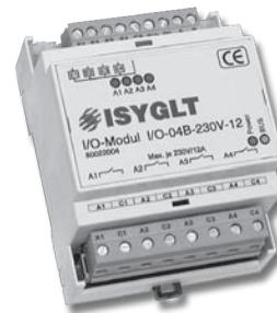
potential available. The functions of all the inputs and outputs can be freely programmed using the software
