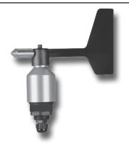
11,25 ° - see technical data). The electrical signals are supplied according to the actual position of the wind vane. The instrument is made of corrosion-resistance material (plastic) and the aluminium parts are additionally protected or varnished resp. by means of an anodic coat. Labyrinth sealing protect sensitive parts inside the instrument against humidity
