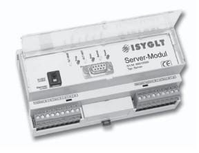
"ProgrammDesigner" (ProgrammDesigner is the programming software for the ISYGLT BUS system), transferred to the master via a programming interface (RS-232) and saved there in the program memory. The program memory can be written as often as you like and even keeps its data in the event of an operating voltage failure. Up to 128 modules are operated on the master subnet. The programm memory is limited to 8 KByte.
